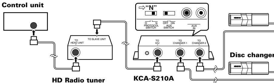
**⚠** Please keep the total extension of the control cable from the control unit to the disc changer to 13 m or less. Control cable lengths in excess of 13 m will cease to function properly.
